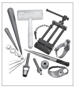
Splicing tools (marlin spike, wooden fid, sewing mallet, splicing clamp) to prepare ropes for or keep them in use. Eyelets, hole punchers and die cutters, needles, special gloves, for keeping protective covers in good order.
