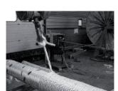
At the beginning of the seizing: Pull the loop underneath the seizing by hand or with the help of a lifting device
