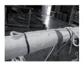
Put a loop parallel on the rope and prelimenary fix with tape
