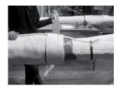
Wind the seizing rope around the rope
