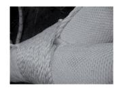
At the beginning of the seizing: Pull the loop underneath the seizing by hand or with the help of a lifting device
