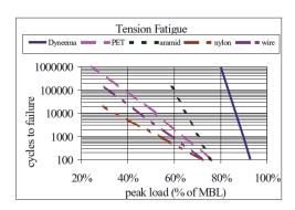
Therefore evaluating the rope damage can primarily assess Safe Working Life of the rope. As a guideline the Residual Breaking Strength of the damaged rope should not be less than 75 % of the New Breaking Strength. Consequently, the number of cycles (for example in an off-loading situation; tanker discharges) are expected to be the main driver for rope disposal. However, this principle should be well understood.
