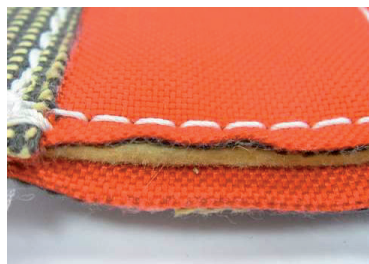
Pic 3: Aramid felt & Red Cordura inner layer
