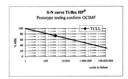
Therefore evaluating the rope damage can primarily assess Safe Working Life of the rope. As a guideline the Residual Breaking Strength of the damaged rope should not be less than 75 % of the New Breaking Strength. Consequently, the number of cycles (tanker discharges) are expected to be the main driver for mooring hawser disposal. However, this principle should be well understood.
