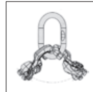
Master link TG 4 4-leg with shortening device Nominal chain dia. 6 to 20mm WLL 3,1 to 33,6 t
