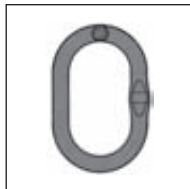
Master link MF Nominal chain dia. 6 to 22mm (1-leg) 6 to 20mm (2-leg) WLL 1,25 to 25 t
