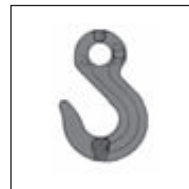
Grab hook GG Nominal chain dia. 7/8 to 19/20mm WLL 2 to 12,5 t
