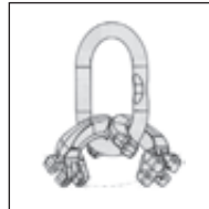
Master link assembly TL4 3-leg without shortening device Nominal chain dia. 6 to 16mm WLL 3,15 to 21 t
