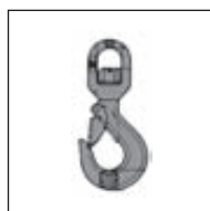
Swivel latch hook LKN with swivel and safety latch Nominal chain dia. 7/8 to 16mm WLL 2 to 8 t
