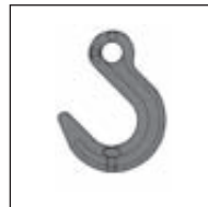
Foundry hook OKE Nominal chain dia. 7/8 to 18/20mm WLL 2 to 12,5 t
