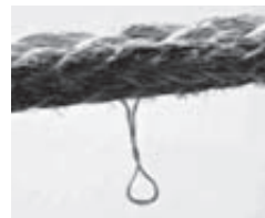
No damage. Single pulled out yarn. Repairable.
