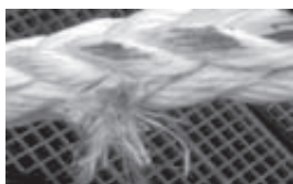
Knotted yarn (inevitable during production of strands). No damage.
