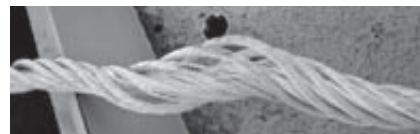
No damage. Single pulled out yarn. Repairable.
