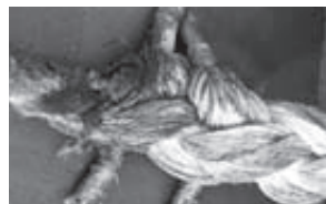
Damaged splice. Irreparable without cutting short.
