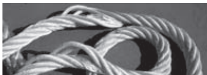
Used rope. Furry surface. No damage.
