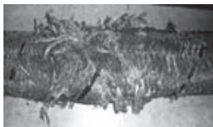
Damaged braided jacket. Repairable if core undamaged.
