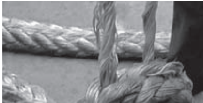
Complete strand pulled out.
