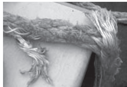
More than 50% of all yarns in one strand cut.
