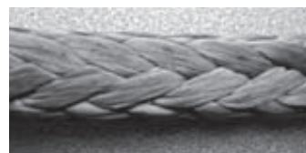
Rope compressed upon heavy load on winch drum. No damage.
