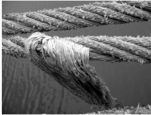
Figure 11: Several inner core yarns pulled out
