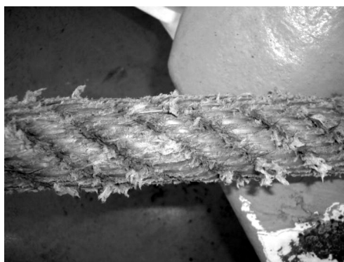
Figure 2: Atlas® Rope with normal abrasion
