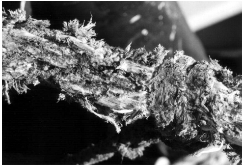
Figure 7: Rope with severe friction burns
