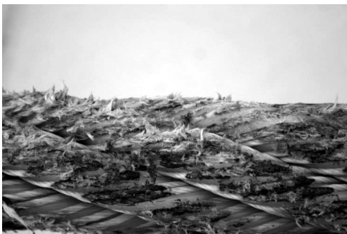
Figure 5: Atlas® Rope with normal abrasion and grease
