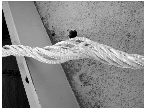
Figure 9: Birdcage in a Atlas® rope
