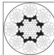
The rope weight is defined as the approximate calculated length mass kg/m (informative). The rope grade is the acronym for the nominal tensile strength of the wires in N/mm<sup>2</sup>. The permitted deviation of the rope diameter from nominal diameter depends on rope type and rope diameter, is normally lower than comparable standard rope.
