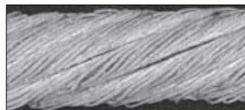
The outer wires wave and the lubricant has completely dried out.
