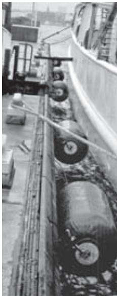
with foam filling, PU coated surface, optionally with chain-tyre net jacket for extra surface protection
