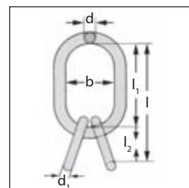
Measurements l<sub>1</sub>, b, and d, refer to sub-links, and apply correspondingly to L, B, and D. The nominal chain diameter refers to use of hook with grade 80 lifting chain lifting sling. WLL β = 0° - 45° (β = tilt angle).
