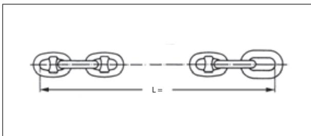
13 Length: One enlarged stud link and studless end link
