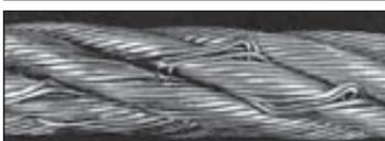
Rope twisted in lay direction. In unloaded condition rope forms a loop in the counter lay direction. If rope is now strained it will be permanently deformed.
