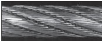
Heavy mechanical abrasion. In spite of high diameter loss (up to 50%) no fatigue breakage. Flattening has increased the contact surface.
