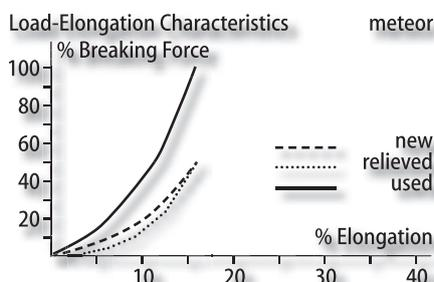
Two examples: Popular rope constructions for anchorages, light and handy. 'Meteor' – low cost, low elongation, for normal requirements; 'Comet' – extremely high tensile strength, extremely low elastic and plastic elongation, for extreme requirements.
