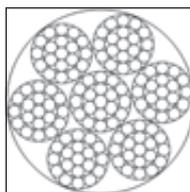
Good runner and rust protection... Flexible, elastic, runs on winches and pulleys, extremely corrosion resistant. But: limited long-term flexural stability.
