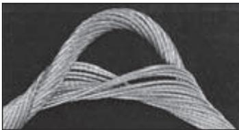
Rope twisted in counter lay direction. In unloaded condition rope forms a loop in the lay direction. If rope is now loaded it will be permanently deformed.
