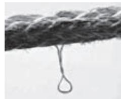
No damage. Single pulled out yarn. Repairable.
