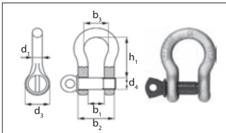
Working Load Limit = 1/6 Breaking Force
