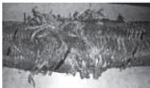
Damaged braided jacket. Repairable if core undamaged.
