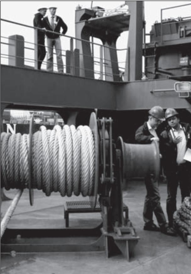
Hence the positioning and specifications of winch drums, rollers and chocks must satisfy requirements of mooring ropes in terms of size, flex, dynamic load properties and material. Efficiency and life of ropes depend critically on how rope guiding equipment and winches, in particular automatic winches, are conditioned, controlled and maintained.
