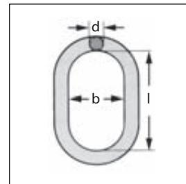
WLL figures shown refer to single leg use. Chain diameters shown refer to use with grade 80 lifting chains.
