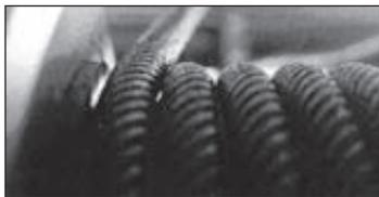
The fleet angle causes segments of the rope being wound onto the drum to rub against the lay on the neighbouring rope causing severe abrasion and twist.
