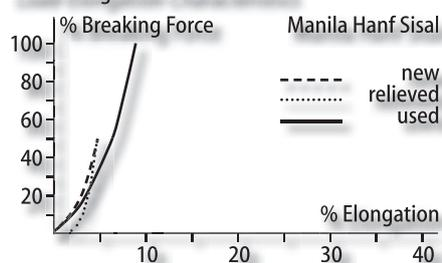
The rope weight is defined as the linear rope mass under pretension. Hemp: 6-14mm +10%, 16-40mm +5%. Permissible limit deviation manila and sisal: 6-8mm ±10%, 10-14mm ±8%, above these ±5%. The nominal rope size is the approximate rope diameter in mm. Minimum breaking forces determined according to current ISO standard. (Test result meets requirement if break occurs either at 100% of relevant value when linear (unspliced), or minimum 90% at splice).
