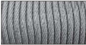
The wear pattern on multi layer drum is indicative of an unsuitable rope diameter.
