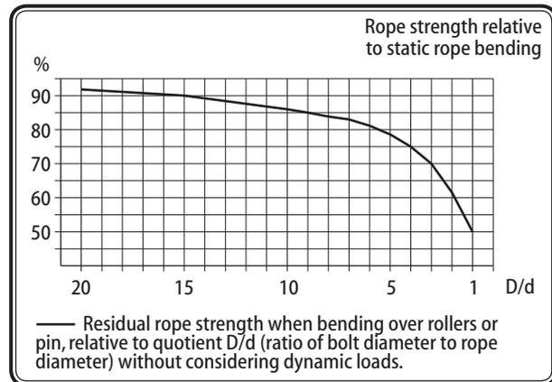
The bend diameter should, depending on material and construction, be adequately large, certainly no less than 5d for fibre ropes made from polypropylene, polyamide and polyester; 8d for wire ropes made from polyamide (d=nominal rope diameter). In ropes made from high modular polyethylene or aramid the bend radius primarily depends on the rope construction, therefore the manufacturer or supplier should be consulted. Sharp edges must at all times be avoided, if necessary by using edge protection.
