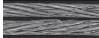
Heavy bending caused the number of internal wire breaks to become visible.
