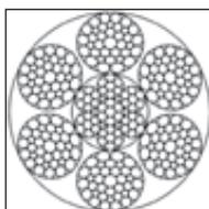
The rope weight is defined as the approximate calculated length mass kg/m (informative). The rope grade is the acronym for the nominal tensile strength of the wires in N/mm<sup>2</sup>. The permitted limit deviation of the rope diameter from nominal diameter is +8-0% for 2 to <4mm, +7-0% for 4 to <6mm, +6-0% for 6 to <8mm and +5-0% for 8mm and more.
