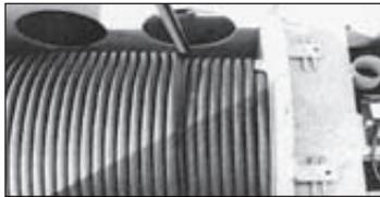
This rope is spooling onto a multi layer drum with special grooving. It is about to cross over one wrap.
